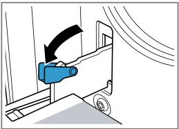
**3.** Close the oven door as far as the limit stop. Grip the left and right hand sides of the door with both hands. Close the door slightly more and remove it.
