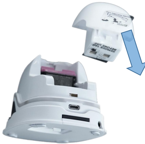
Fig. 9: Battery contact insulating tape
