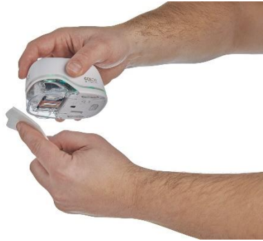
Fig. 28: Clean print head with damp cloth
